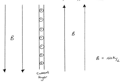
The field strength is given by  $B_{K(in)} = \mu_o K/2$  (on the right hand side of the sheet) and  $B_{K(out)} = -\mu_o K/2$  on the left hand side of the sheet. Hence to find the total magnetic field just inside the magnetopause boundary we need to add the effect of the magnetic field from the current layer to that of the dipole field and so
